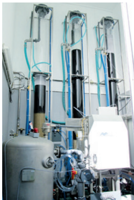
Abb. 4.1: Examination of the adsorptive behavior on granular activated carbon within the joint research project SchussenAktivplus (© SchussenAktivplus)
